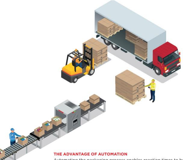
Automating the packaging process enables reaction times to be improved and to synchronise order preparation as near as possible to the departure times of the transporters.
