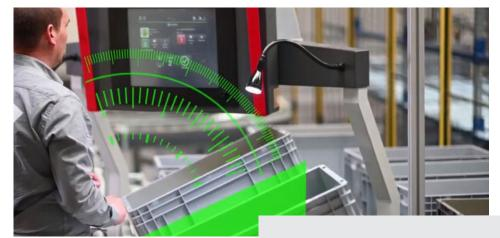
**Tilting of containers:** this system reduces the stresses on the shoulders and on the bust. The operator does not need to bend over to pick or place the products. Movements are thus restricted to the order picker's comfort zone.
