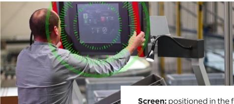
**Screen:** positioned in the field of vision and containing only the information essential to the preparation: the operator does not need to raise their head or make neck movements to access the information. The height and depth of this HMI can be adapted to the operator.
