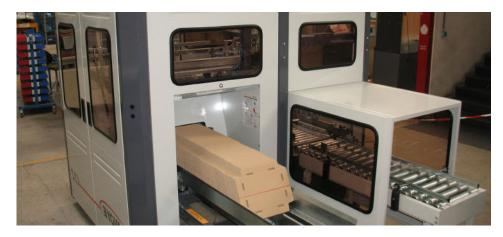
The PAC600 range of secure parcels: these forming machines allow you to design very strong packaging, which is complemented by wedging using a shrink wrap film. Just adding a lid, rather than using flaps, reduces the cardboard area by 10%.
